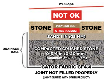
Sand or ASTM No. 9 Stone can be used as a bedding layer
